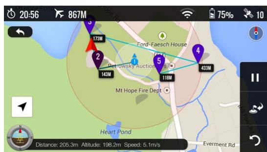
Figura 1. Autopiloto programable DJI Ground Station
